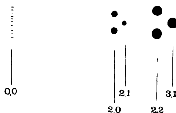
Fig. 4. Theoretical intensity distribution for the suggestion of §7, based on equatorial projections with a dimer model where 2R/a = 0.9 . The 2,2 and 3,1 reflexions of a 3.8 nm square cell are not particularly sensitive to the value of 2R/a chosen. The 2,0 and 2,1 reflexions are sensitive. In particular, for the simple cylinder model used, the 2,1 reflexions disappear if 2R/a = 1 . 'Tilt' in the gap region is \sim 5^\circ . Area of spots is proportional to the calculated intensity.
